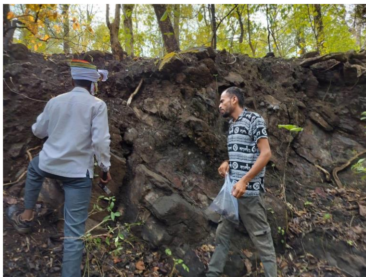
Figure 3: Photograph showing channel sampling at existing trench
